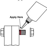
For Blind Holes, apply several drops down the female threads into the bottom of the hole. As threads are engaged, compressed air forces the product upwards into the threads.
